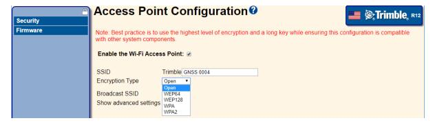
Note: You can view and configure additional access point settings by ticking the "Show advanced settings" checkbox.
