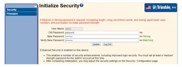
**Note:** If the 'admin' user password is lost, the password can be changed by resetting the receiver to factory defaults. This is done by pressing and holding the physical power button on the receiver for 30 seconds. For receivers with a front panel display, e.g. Trimble R750, you will need to contact Trimble Support via your dealer to obtain a code to reset the password. This is done to prevent unauthorized access to computer networks from a networked receiver.
