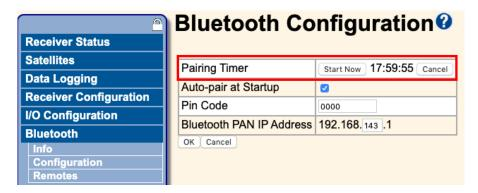
The timer can be also reinitiated without accessing the receiver WebUI by power cycling the receiver. While the timer is active, the *Bluetooth Info* menu will show that the module is discoverable.
