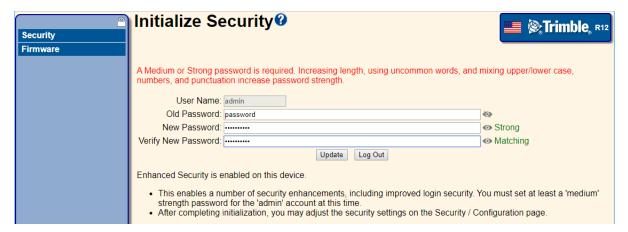
**Note:** If the 'admin' user password is lost, the password can be changed by resetting the receiver to factory defaults. This is done by pressing and holding the physical power button on the receiver for 30 seconds.
