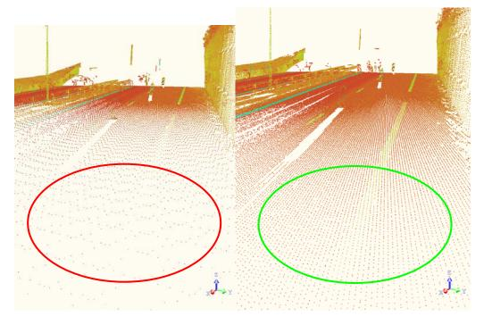
Fig 1. SureScan (right) highlights the increased coverage and uniformity of the data captured on a road surface.
