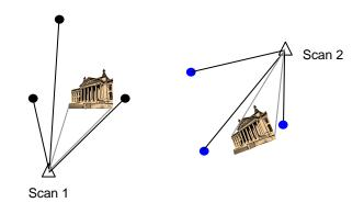
Figure 1: Multiple scans to common targets or spheres
