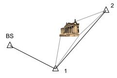
Figure 3: Traditional total station workflow
