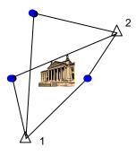
Figure 2: Relating multiple scans to common targets or spheres
