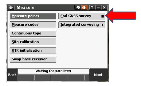
Click END GNSS SURVEY. This will end the ROVER. Select POWER OFF RECEIVER.
