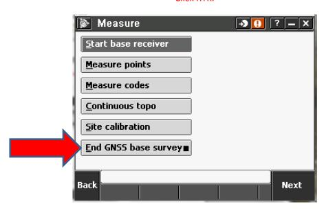
Click END GNSS BASE SURVEY. This will end the BASE. Select POWER OFF RECEIVER.
