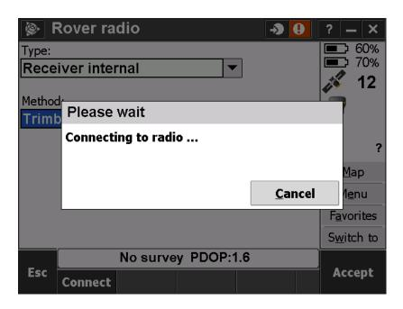
Radio configuration make sure radio operation mode is Rover, Frequency 464.50000 MHz and Base radio mode is TT450s at 8000 bps and hit Enter (Frequencies must match Base as well!)
