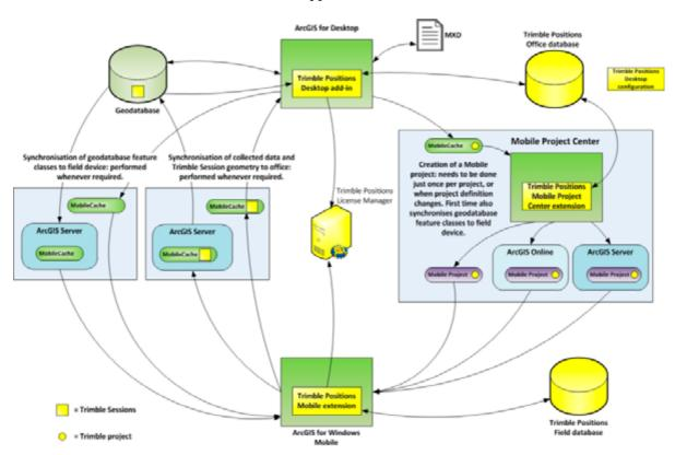
The Trimble Positions Mobile extension allows high-accuracy geometry collection from within the Esri ArcGIS for Windows Mobile data collection application.
