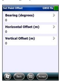
**Note** – The bearing value is always interpreted as relative to True North. The supported laser rangefinders have a configuration option to configure the device with the magnetic declination. Remember to regularly calibrate and configure your electronic compass.
