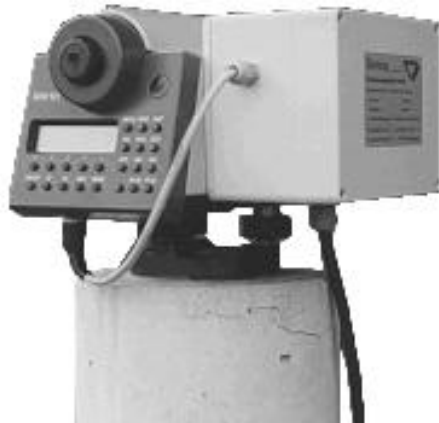
Figure 7: DiNi ® 10T modified for the monitoring of structures
