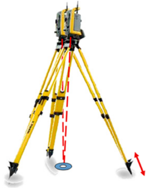
Figure 1: Trimble SurePoint Technology Corrects Leveling Errors in Trimble S-Series Total Stations
