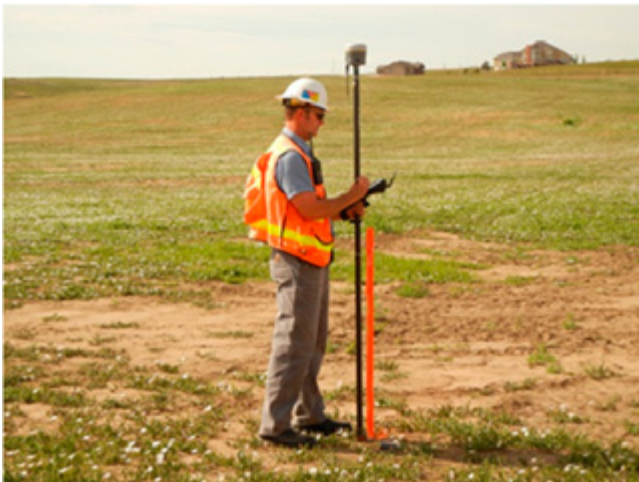
Figure 2: Ground positioning error increases with pole tilt
