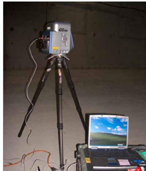
Figure 5: Trimble 3D scanner in tunnel
